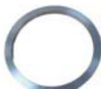
MP-ALKO-RING Ring to convert parallel hubs to alko Insert inside cup of outer bearing in drum
